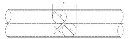
Two holes are drilled at all outlets for optimum emptying. The hole positions should be staggered in relation to one another.
